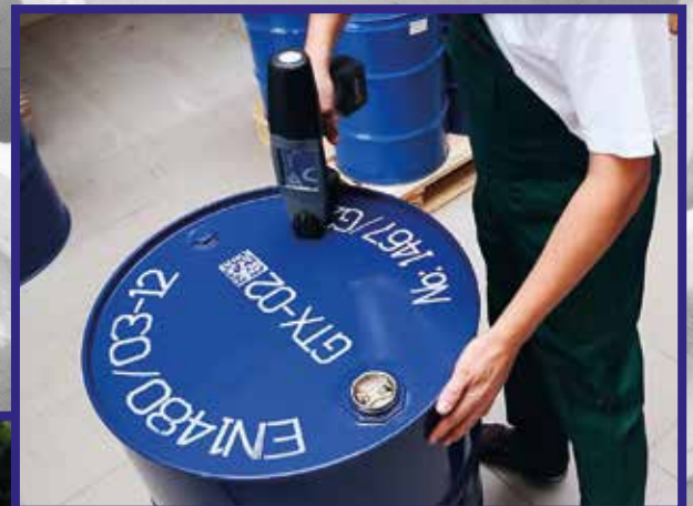
EBS-260 printing Datamatrix code
